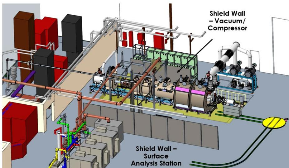
Figure 4-2. Current layout of shield walls relative to MPEX system.
