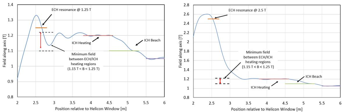
**Figure 3-1: Illustration of magnetic field ripple requirement with respect to the transition between the ECH and ICH magnet subsystems.**
