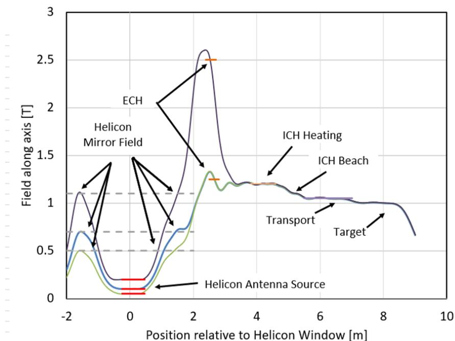
Figure 3-1. MPEX magnetic field profiles for different Helicon and ECH operating modes for 70 GHz baseline configuration.
