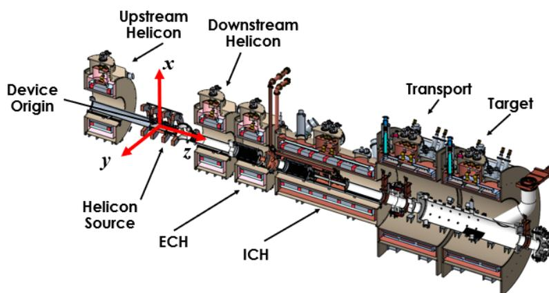
Figure 1-2: Illustration of device origin and reference axes relative to cross section of MPEX magnet systems.
