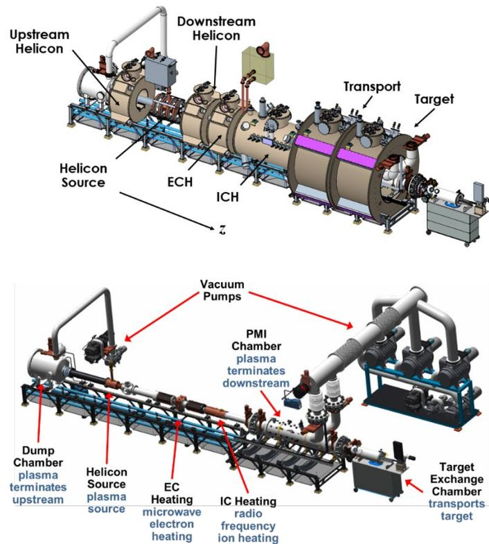
Figure 1-1: Current design for MPEX with (top) and without (bottom) the magnet system illustrated along with other MPEX system and components.
