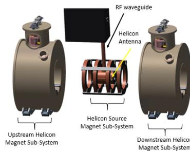
Figure 4-3. Layout of Helicon Magnet Sub-systems with an emphasis of the axial clearance needed for the Helicon Source Magnet Sub-System relative to the RF waveguide.
