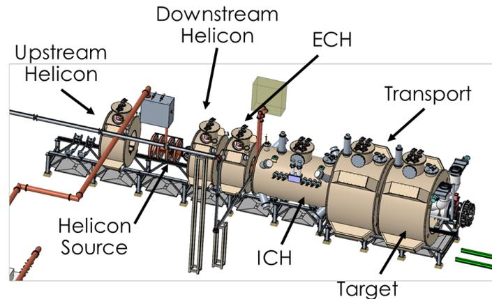
Figure 4-1. Rendering of MPEX magnet system based on reference design [2].
