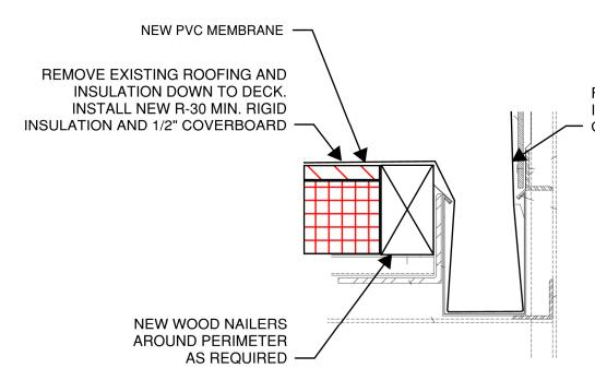
FULLY ADHERE NEW MEMBRANE TO INTERNAL GUTTER. WRAP UP AND OVER PARAPET, UNDER COPING
