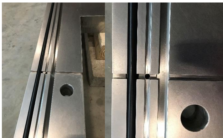
Figure 2.5 – Example of o-ring groove with vent groove
