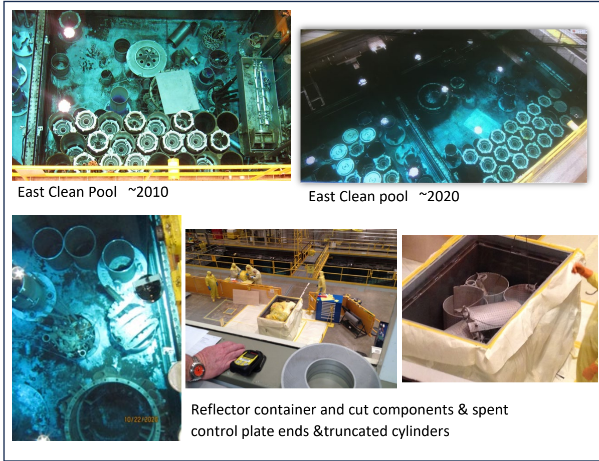
Figure 7 Examples of radioactive and mixed waste stored at HFIR to be disposed of by Subcontractor.
